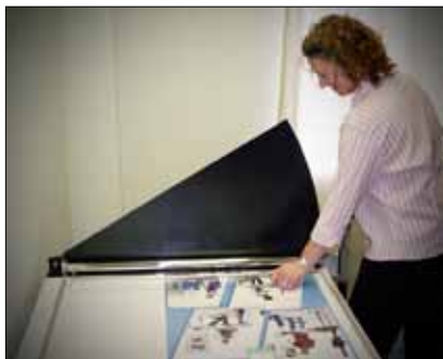
Manual clamping system holds work securely in place and prevents fanning
